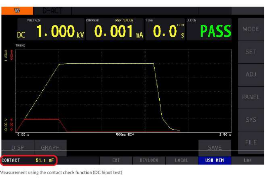
Measurement using the contact check function (DC hipot test)
